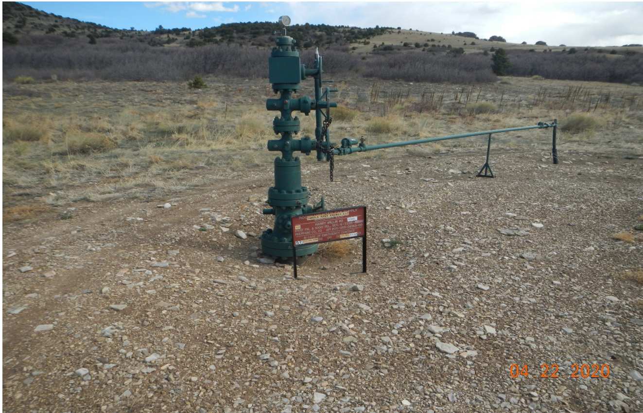
Photo 3. Well sign is posted at the well head. Emergency contact number on the sign needs to be updated.
