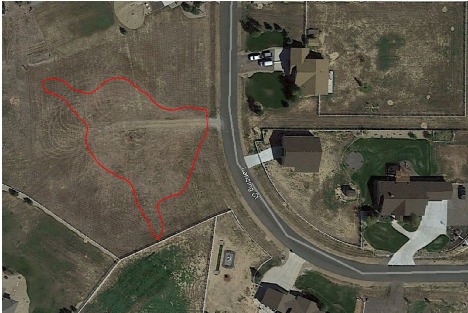
Photo 1. Google Earth aerial imagery taken 9/12/2019 illustrating the approximate damage due to vehicle rutting. The approximate area illustrated in red was mapped on 4/8/2020 using a Trimble Juno 3B handheld device.
