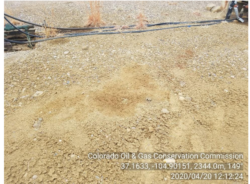
PHOTO 8: AREA OF IMPACTED SOIL NEAR HYDRAULIC HOSED BETWEEN ENGINE SKID AND WELLHEAD. Conduct maintenance on equipment, cleanup stained material and review self inspection processes. CA DATE 4-25-20.
