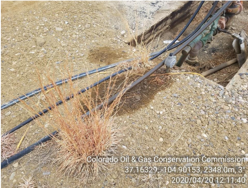
PHOTO 7: AREA OF IMPACTED SOIL NEAR WELLHEAD APPEARS TO BE FROM HYDRAULIC HOSED. Conduct maintenance on equipment, cleanup stained material and review self inspection processes. CA DATE 4-25-20.
