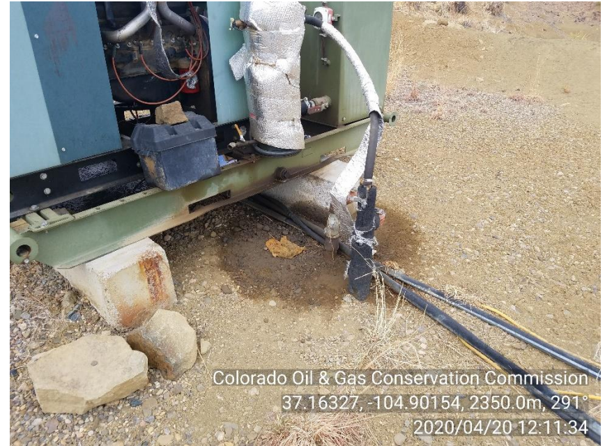
PHOTO 8: AREA OF IMPACTED SOIL AROUND ENGINE SKID. Conduct maintenance on equipment, cleanup stained material and review self inspection processes. CA DATE 4-25-20.
