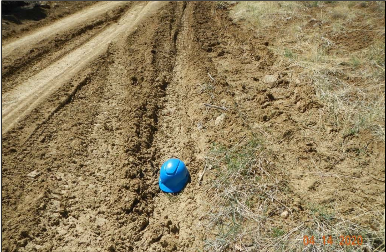
Photo 4. View of deep rutting (approx. 1.5 ft deep) and evidence of vegetation damage along the access road.
