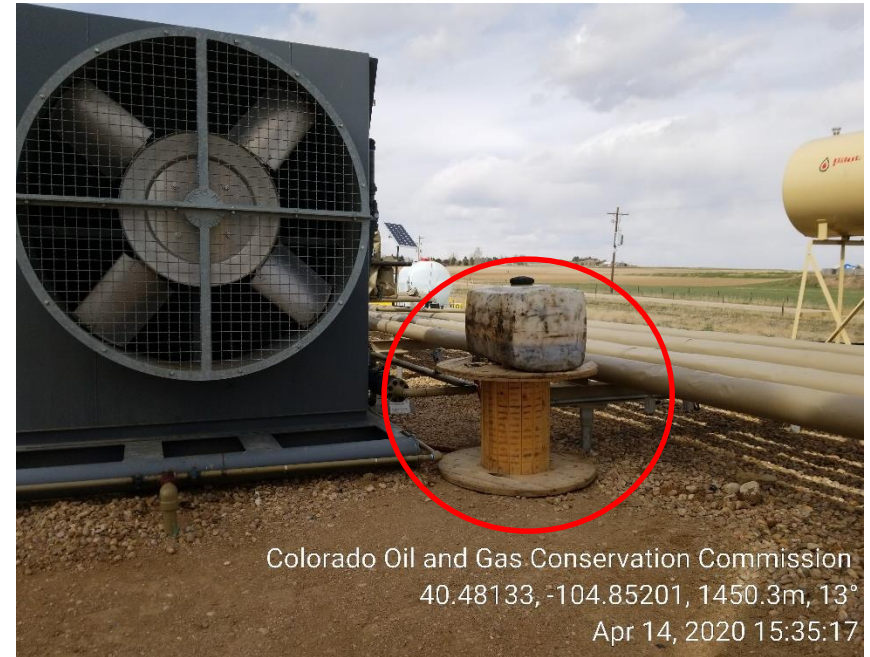
Photo 14: Container not in containment
