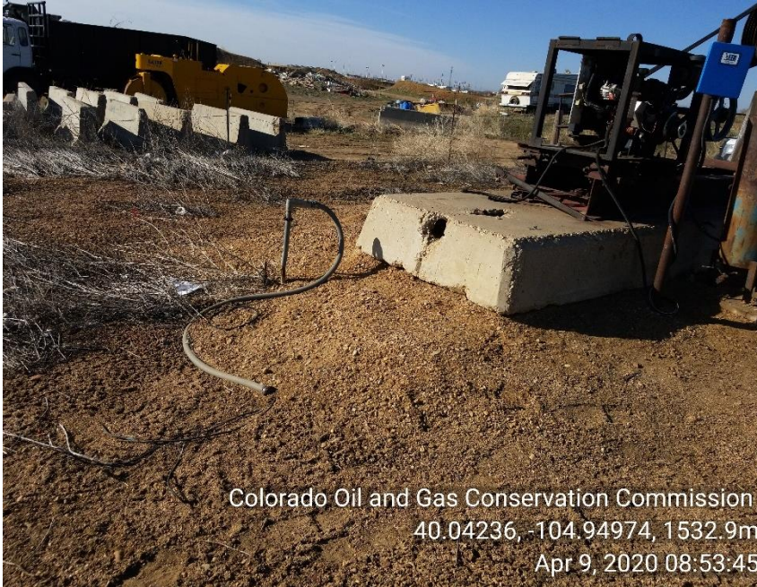
Photo 3 unused equipment: Unused electric line with exposed wires not marked not LOTO. As you can see in photo gas powered motor has been installed no electric motor.
