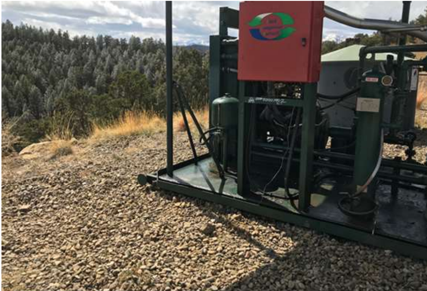
PHOTO 5: THE OIL ACCUMULATION ON THE SKID WAS REMOVED AND THE SOIL/GRAVEL WAS CLEANED UP.
