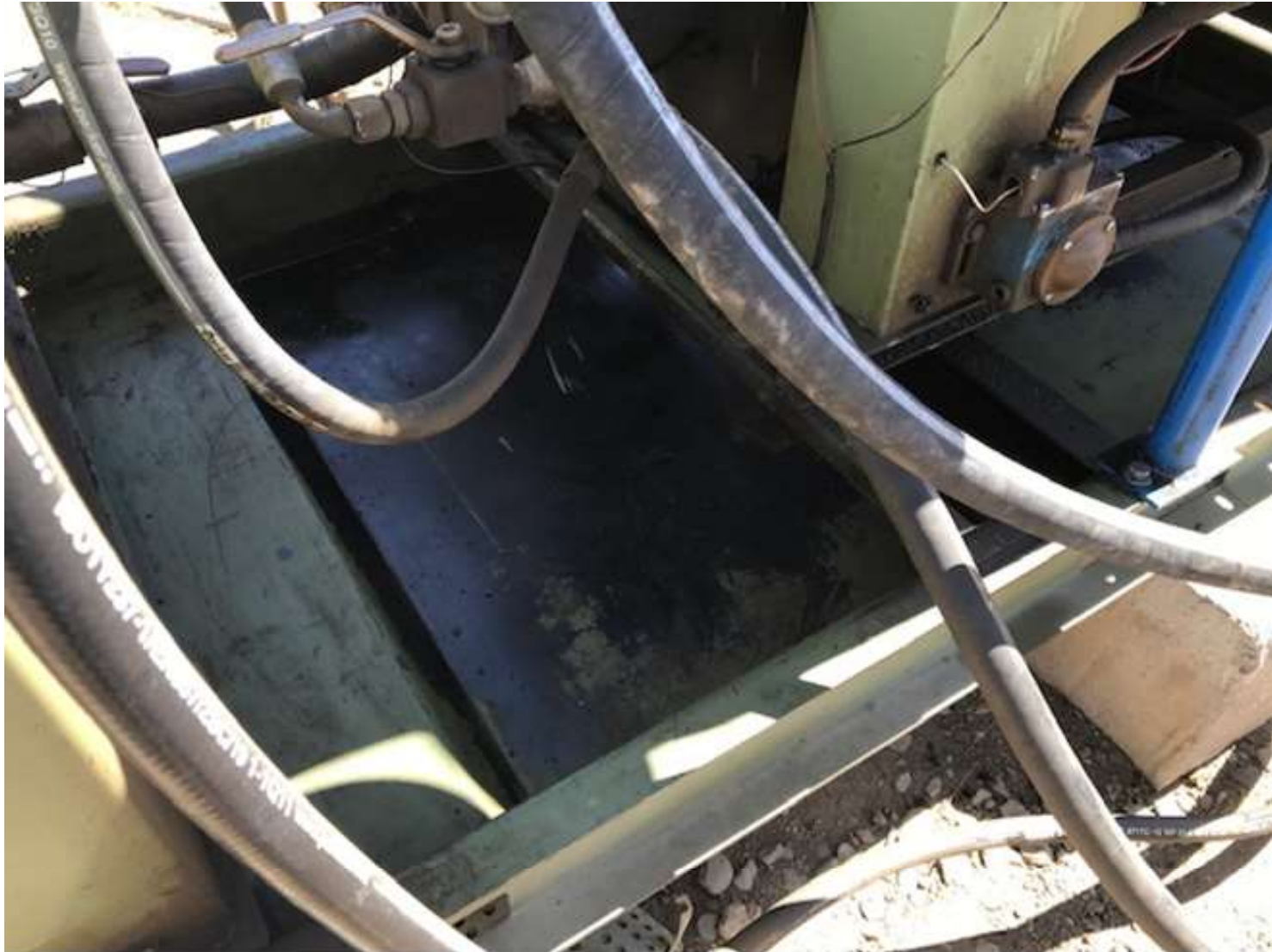
PHOTO 2: THE OIL LEAK ON THE ENGINE SKID WAS REPAIRED. THE OIL ACCUMULATION ON THE ENGINE SKID WAS REMOVED AND THE SKID WAS CLEANED.
