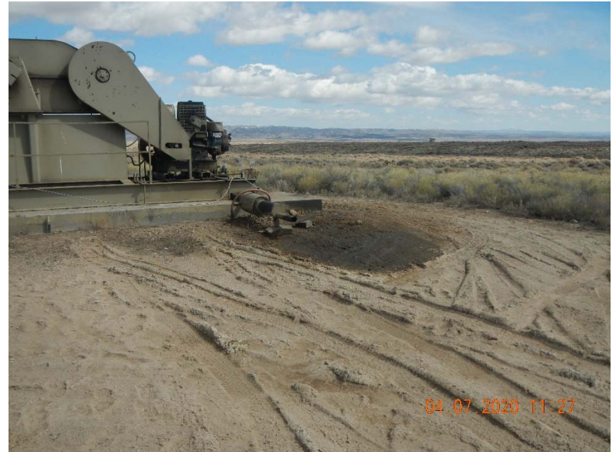
Photo 6. Stained soil at pump jack.
