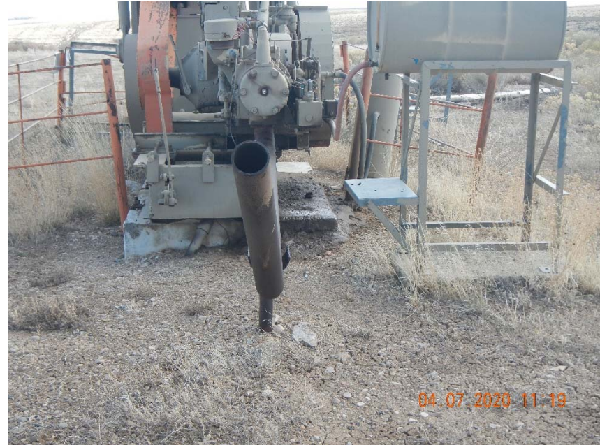
Photo 3. Stained soil on right side of pump jack.
