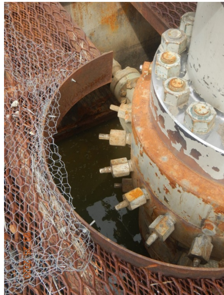
Photo#6: Cellar grates (covers) are not complete.
