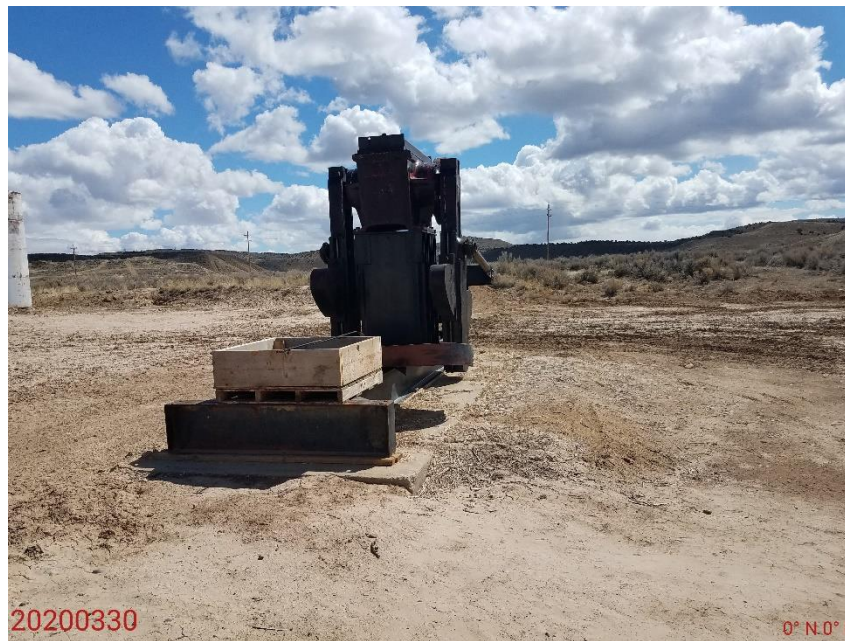
Photo 6: Photo taken from the well site, facing south. Photo shows well appears to have been plugged; Pumping unit remains on the Location.
