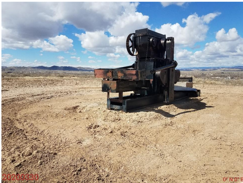
Photo 5: Photo taken from the well site, facing northwest. Photo shows well appears to have been plugged; Pumping unit remains on the Location.
