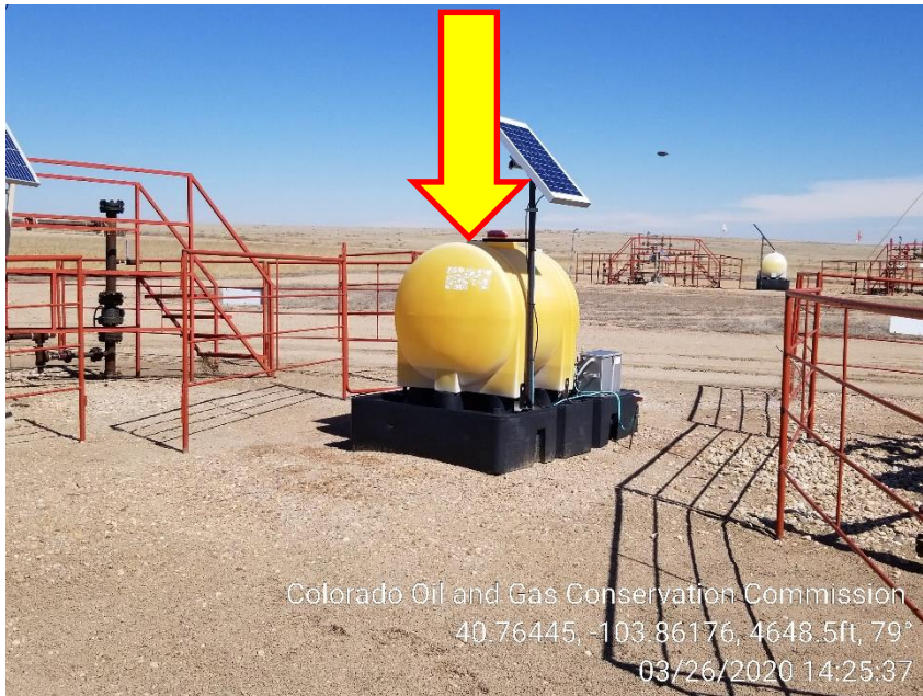
Photo 9 – Westside Chemical tank – missing/faded Label
