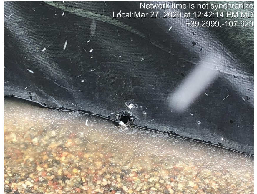
Photo #0855 Hole in tank containment liner.
