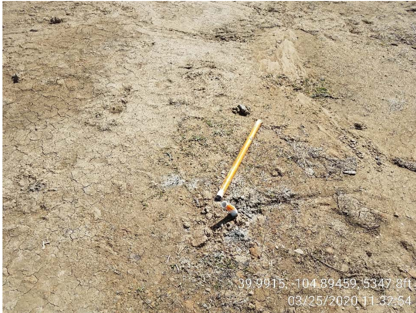
Photo 5 – Damaged monitoring well within fenced area.
