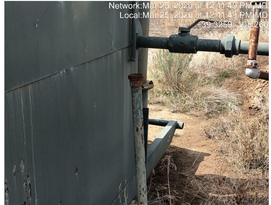
Photo #0820 Flow line risers not LO/TO.
