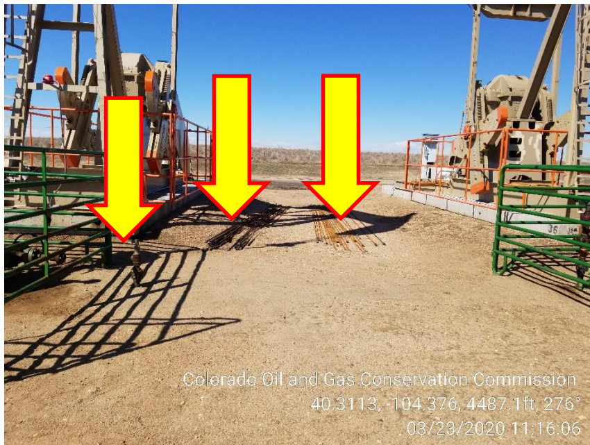
Photo 7 – Unused Rods, Unmarked Riser
