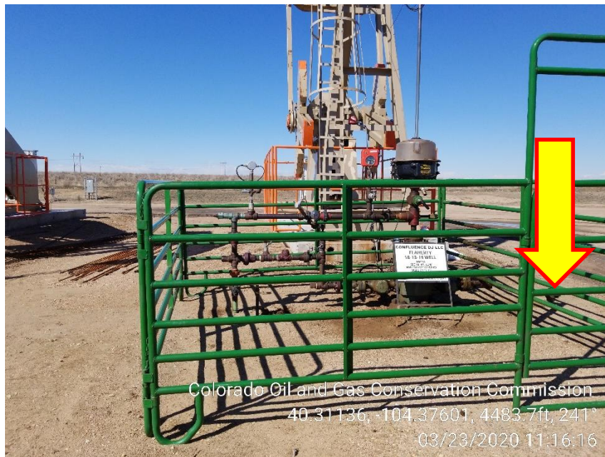
Photo 5 – Stained Soil at Wellhead, Unmarked Riser
