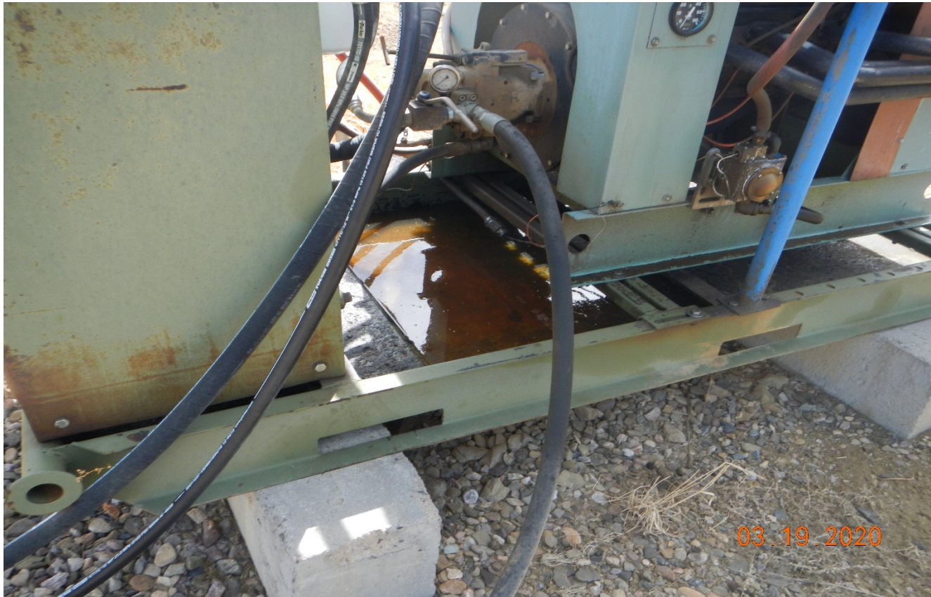
Photo 8. The oil on the engine skid on the other engine skid that needs to be cleaned up.
