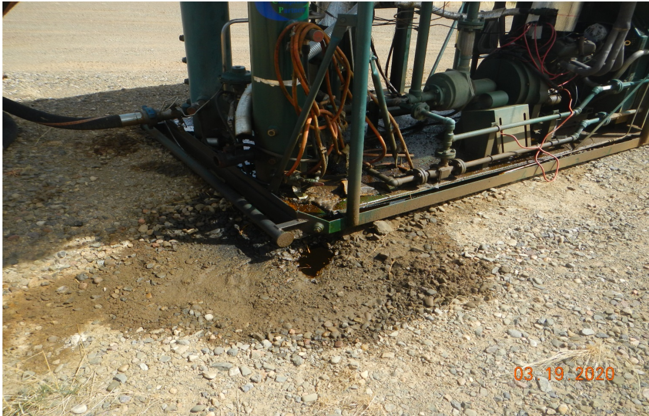
Photo 7. There is oil stained soil and oil on the engine skid that needs to be cleaned up.
