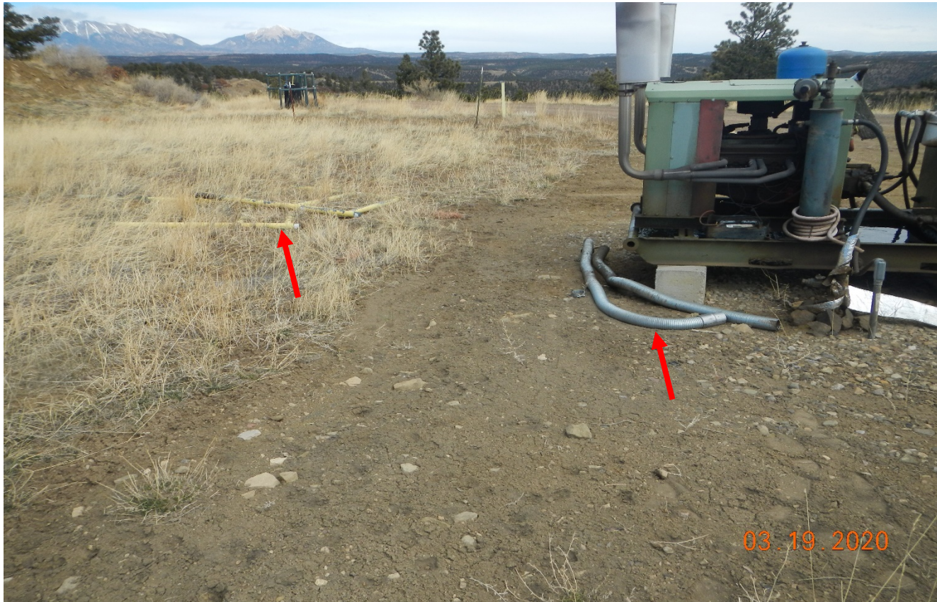
Photo 4. The exhaust pipe is laying on the ground and pipe h braces guards are laying in the grass. Unused equipment needs to be used or removed.
