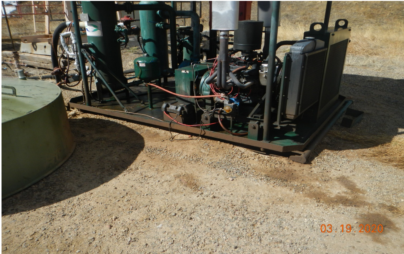
Photo 6. The oil in the engine skid has been cleaned up. There is still some spotting stained soil around engine skid.
