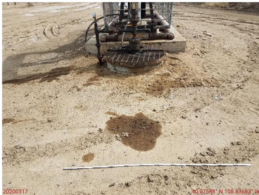
Photo 5: Photo taken from the wellhead, facing east. Photo shows stained soils around the well. 6 foot measuring stick for reference.
