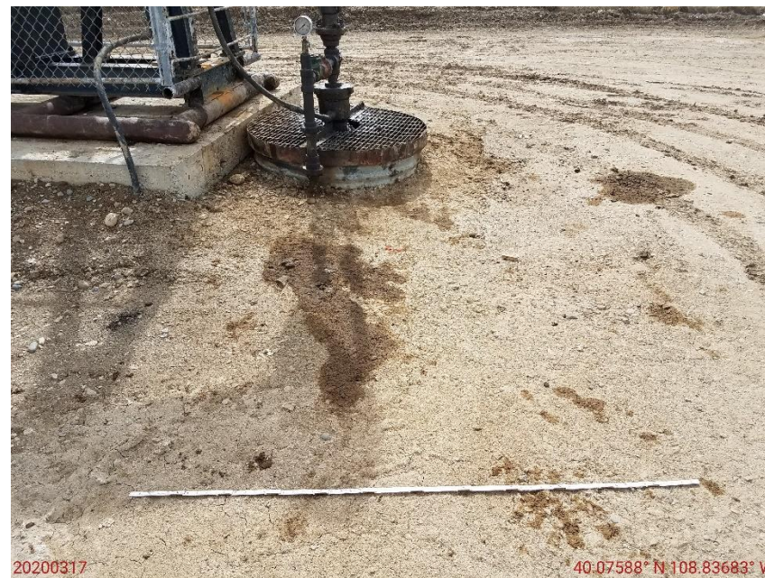
Photo 4: Photo taken from the wellhead, facing south. Photo shows stained soils around the well. 6 foot measuring stick for reference.
