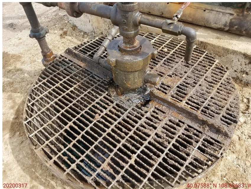
Photo 6: Photo taken at the well head. Photo shows containment cellar; various chemicals/fluids appear to have discharged into the containment BMP; chemicals/fluids require removal. Photo also shows various chemicals/fluids on the well/casing
