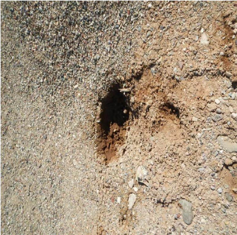
Photo#2: Hole developing in containment.
