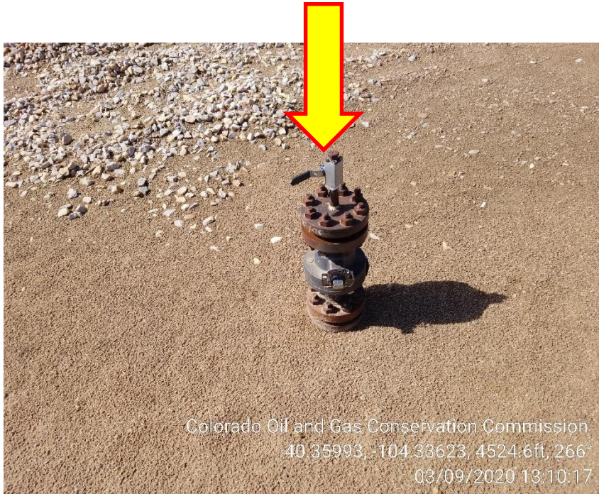
Photo 5 – Unmarked Riser
