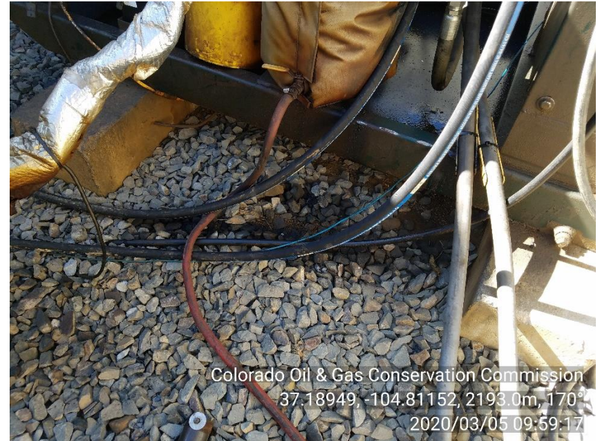
PHOTO 8: IMPACTED SOIL/GRAVEL NEAR PRIME MOVER ENGINE SKID. Conduct maintenance on equipment (ie REPAIR LEAKS ON ALL EQUIPMENT), cleanup stained material and review self inspection processes. CA DATE 4-5-20
