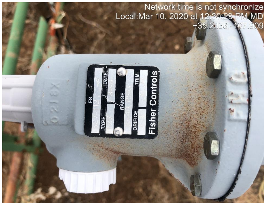
Photo #0744 Pressure plate of Little Joe regulator.
