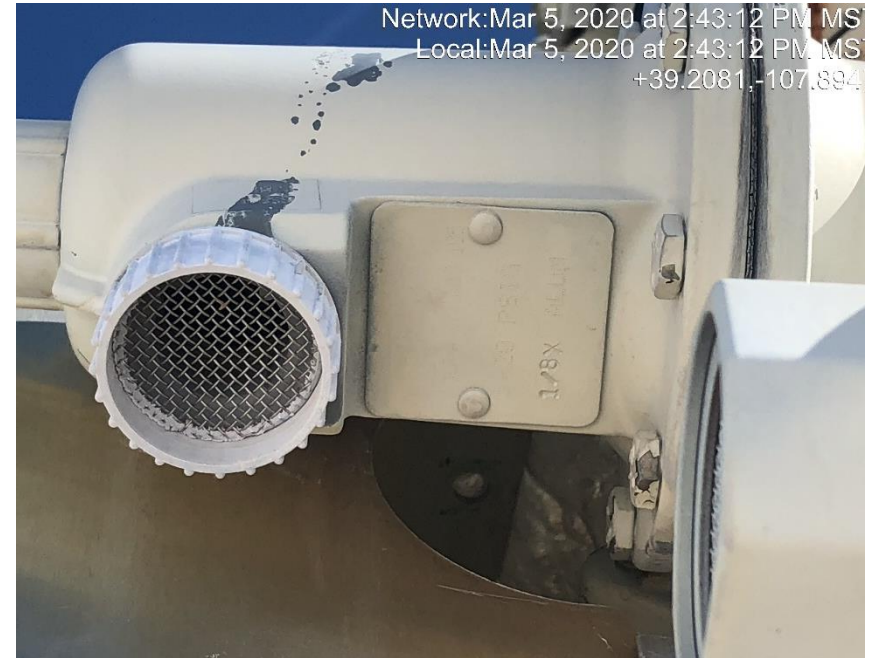
Photo #0712 Pressure plate of secondary regulator.
