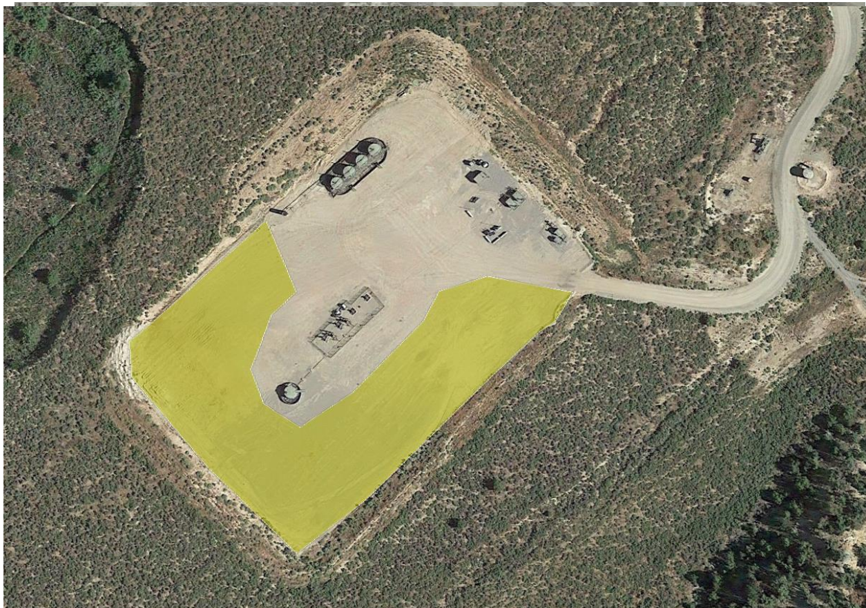
Photo 61: 2019 Google Earth Aerial imagery. 2A #400820779 states size of Location post interim reclamation to be 2.67 acres. Photo shows Reclamation Specialist measured the area of the current production area, including stormwater BMPs via a Trimble handheld GPS unit; The current production area is 4.5 acres in size. Interim reclamation has not been conducted. Photo shows areas on the west, south and eastern ends of the current pad that do not appear to be needed for production activities.
