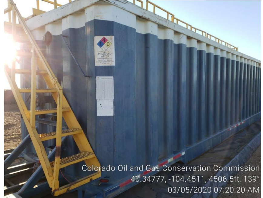
Photo #4 Frac Tank for Sand cans
