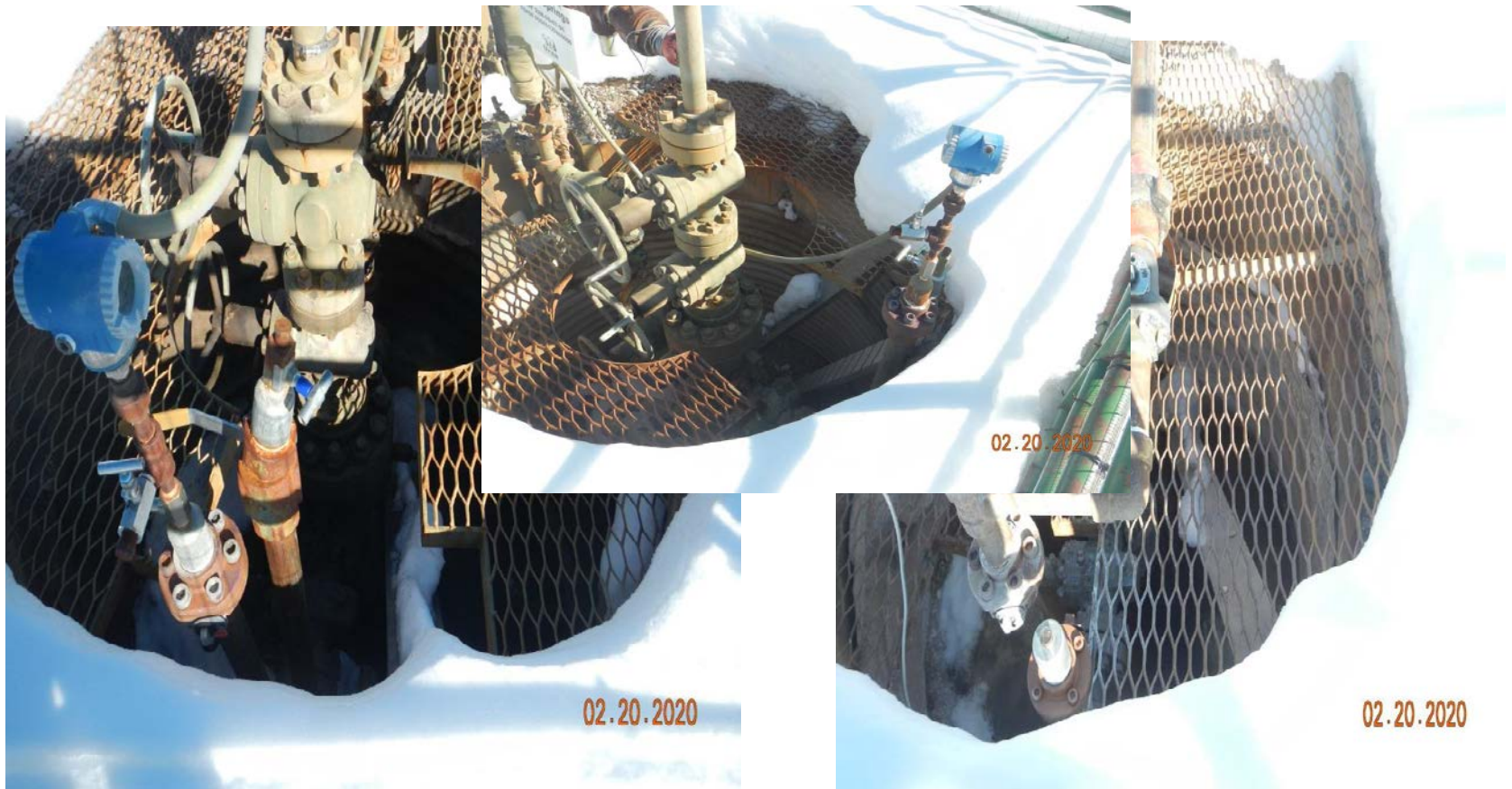
Photo#2: Wildlife Escape Board are improperly adjusted.
