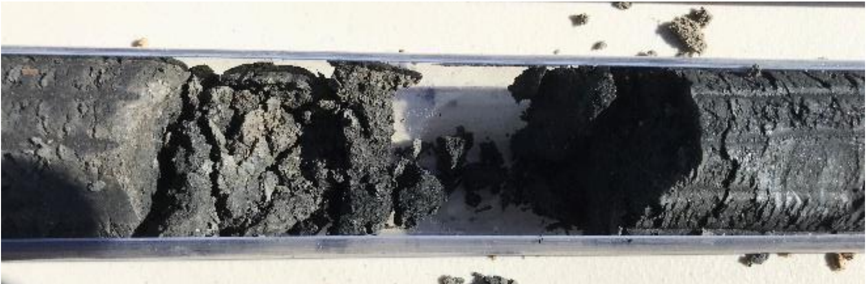
Photograph 1: Typical lithology observed at the BW Musser 11 pad, Pit 3, COGCC ID 100382. Black clayey silt was encountered consistently at all boreholes completed at this pad. Note the black coloration, which was indicative of soil impacts at Pit 3.
