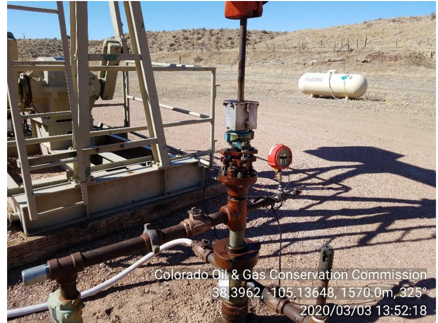
PHOTO 4: Polish rod oiler is running oil down wellhead assembly, This is not a ca notice as oil has not reached the ground. This is just a reminder that if this oil contaminated the soil that would result in a corrective action being administered.
