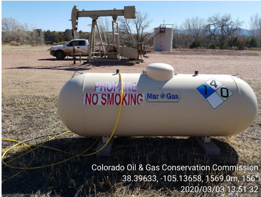
PHOTO 3: unused equipment stored on location (propane tank is not being used). Remove unused equipment per rule 603.F. ca date 4-3-20
