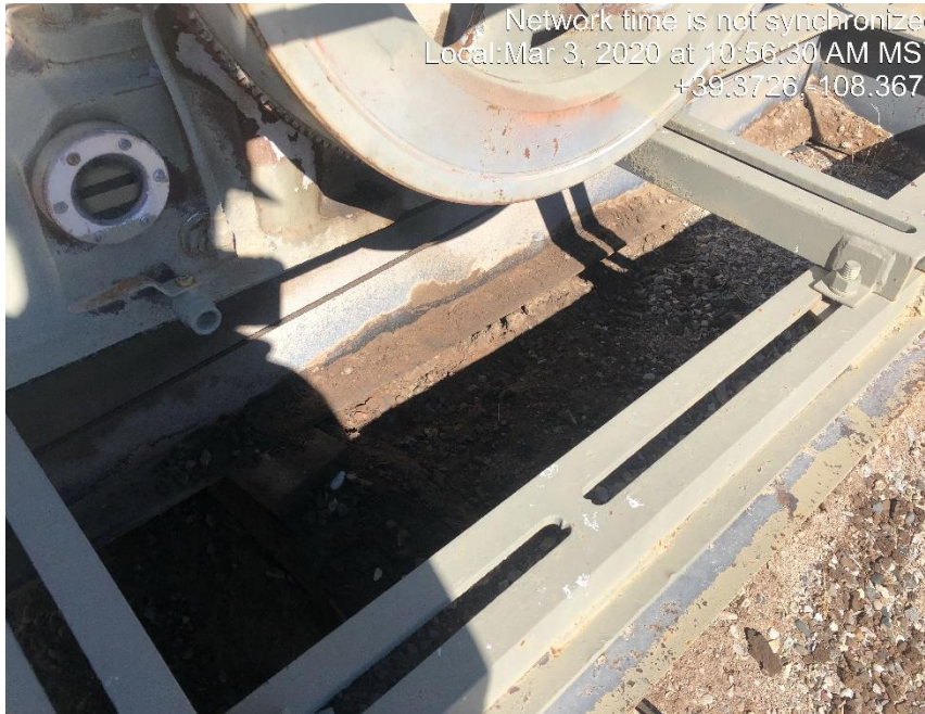
Photo #0682 Stained soils under pump jack.
