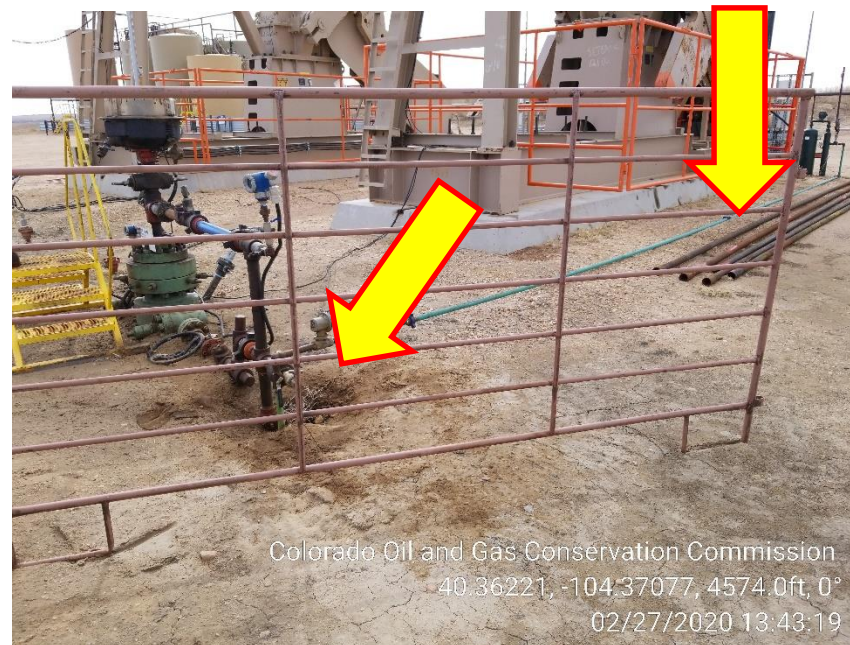
Photo 2 – Stained Soil and unused Tubing Strings at K-O-31
