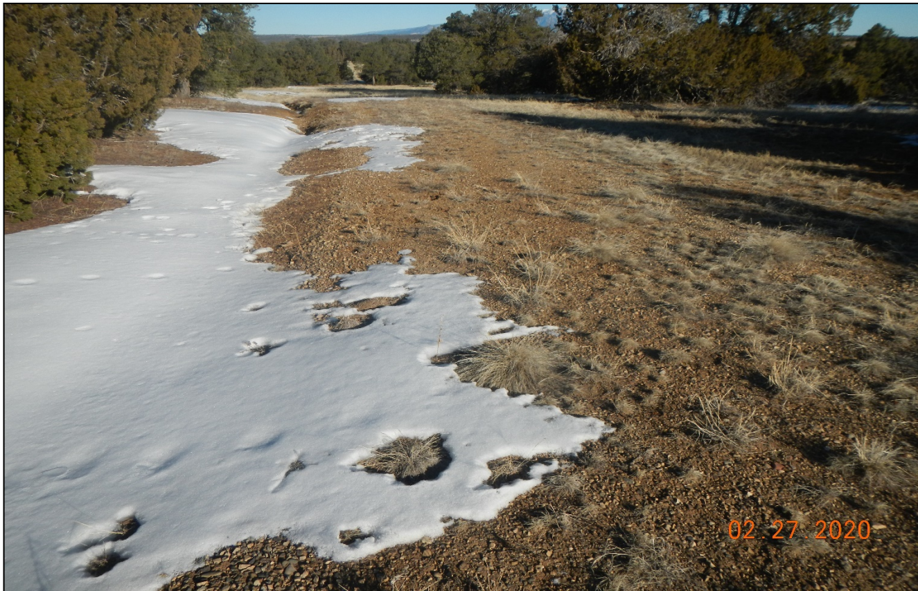
Photo 2. Northwest along the access road. This area is sparse of vegetation. This area may need decompaction and leveling to fill in erosion shown in the next photo.
