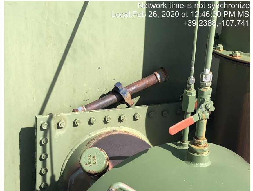
Photo #0648 Unused 1" nipple and wing half on separator burner.
