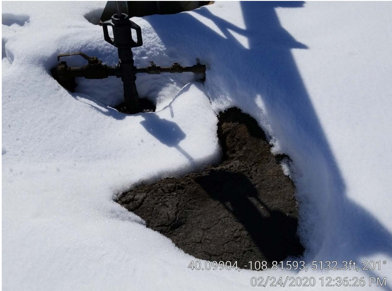
Photo 4. Oily soil next to well Stagner 2.
