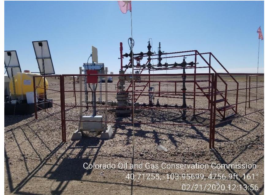
Photo 2 – Haley LC27-715 missing Wellhead Sign
