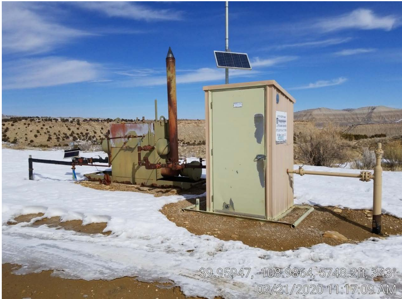
Photo 3. Separator & meter building.
