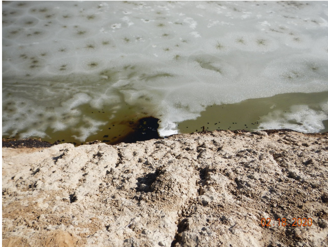
Photo # 3 – Oily soil on pit bank, oil on surface of pit
