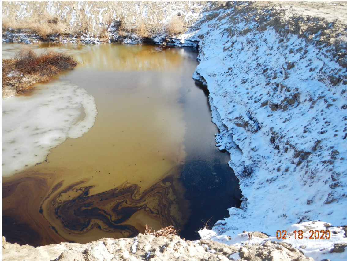
Photo # 4 – Oily soil on pit bank, oil on surface of pit in southwest corner
