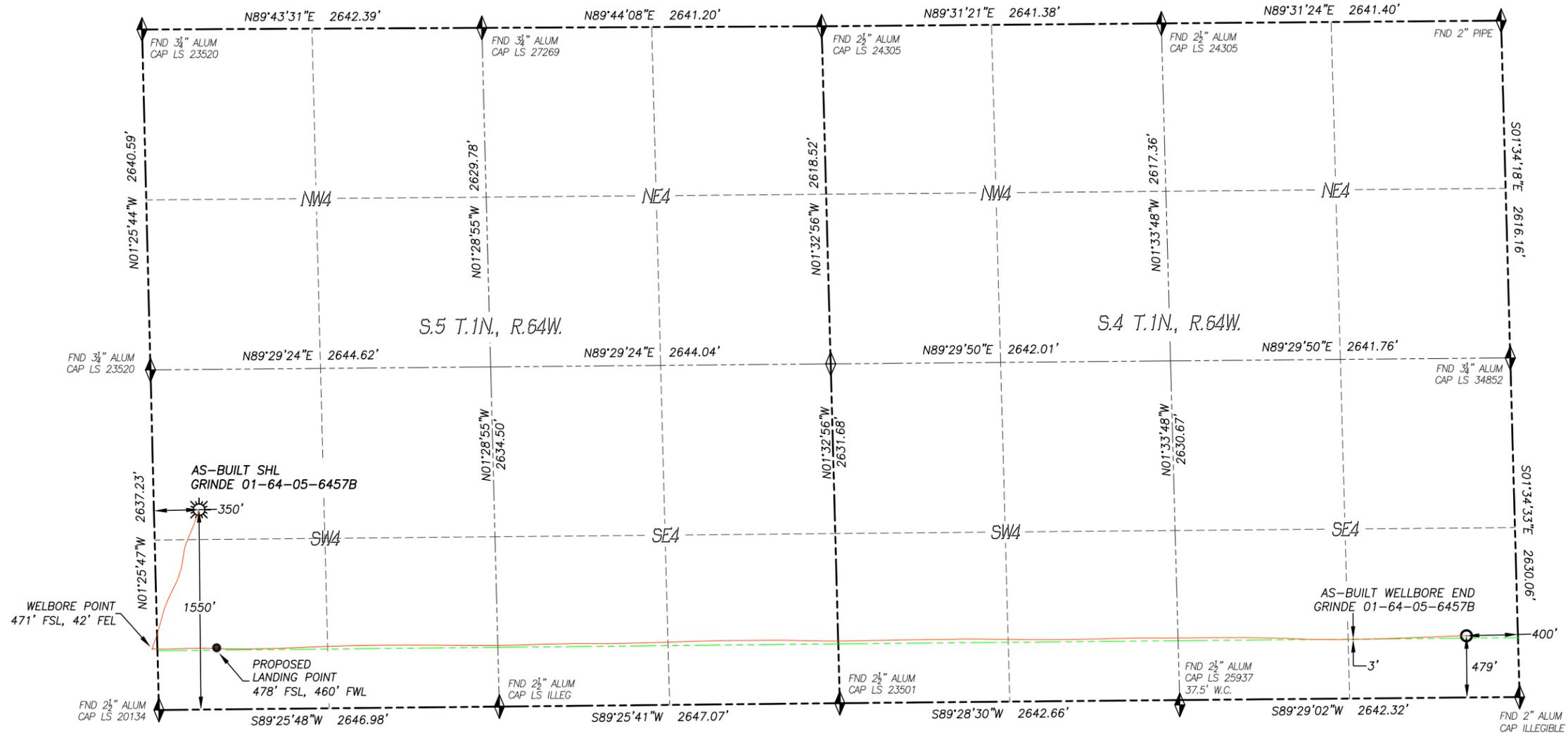
IN ACCORDANCE WITH A REQUEST FROM HIGH POINT RESOURCES, DALEY LAND SURVEYING, INC. HAS DETERMINED THE SURFACE LOCATION OF THE GRINDE 01-64-05-6457B WELL TO BE 1550' FSL, 350' FWL, AS MEASURED AT NINETY (90) DEGREES FROM THE SECTION LINES OF SECTION 5, TOWNSHIP 1 NORTH, RANGE 64 WEST AND THE BOTTOM HOLE LOCATION TO BE 479' FSL, 400' FEL, AS MEASURED AT NINETY (90) DEGREES FROM THE SECTION LINES OF SECTION 4, TOWNSHIP 1 NORTH, RANGE 64 WEST, OF THE 6TH PRINCIPAL MERIDIAN, WELD COUNTY, COLORADO.
