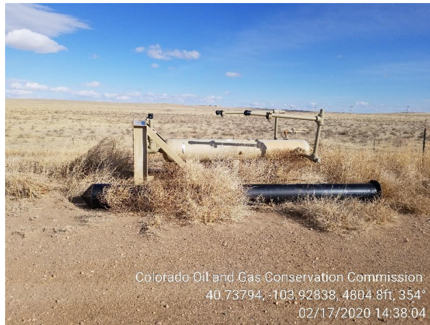
Photo 2 – Unused Sand Trap and Separator Stack in the NE corner of location
