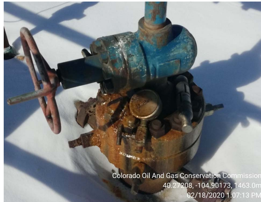
Master valve leak
