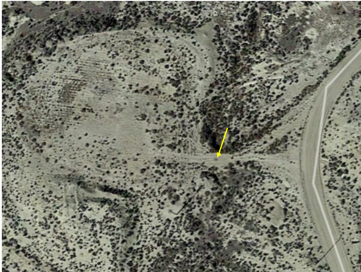
Photo 9: Aerial imagery showing section of access road across a drainage that requires reclamation.
