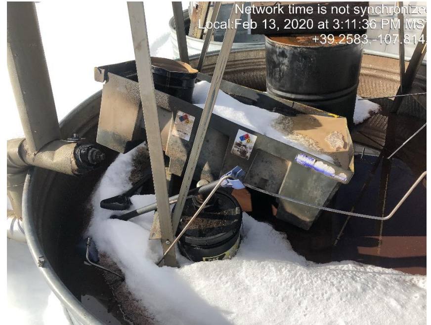
Photo #0593 Used filters and trash inside multiple tank containments.
