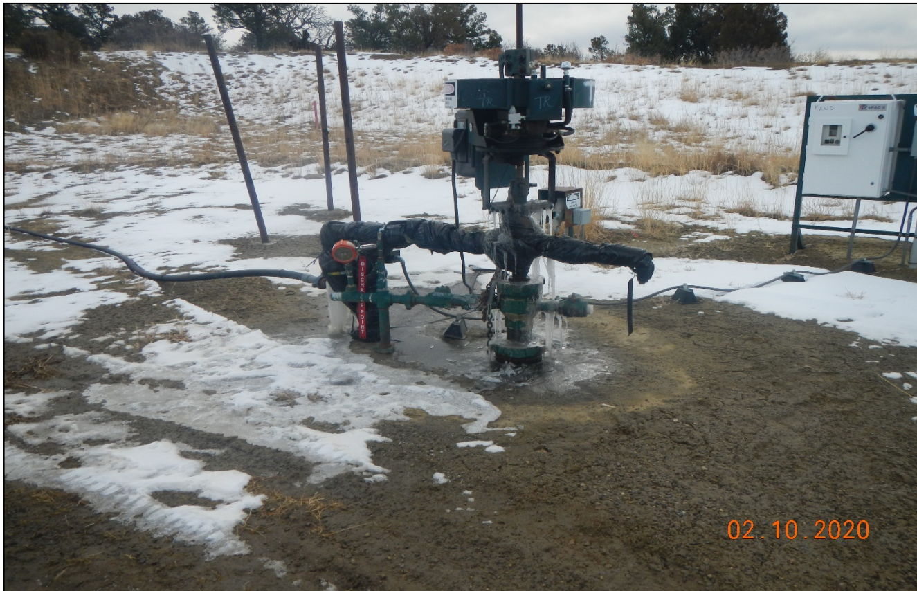
Photo 2. There is a water leak at the PR well which needs to be repaired.
