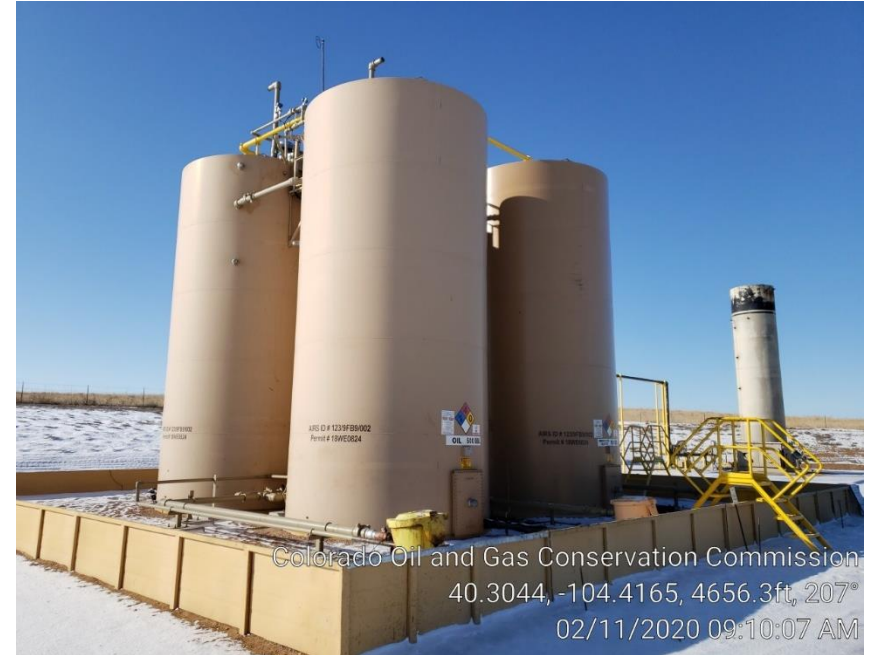
Photo #3 Tank Battery
