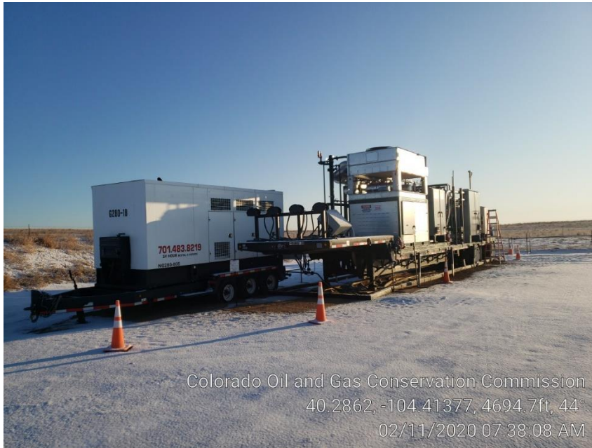
Photo #7 Generator & Dehydrator
