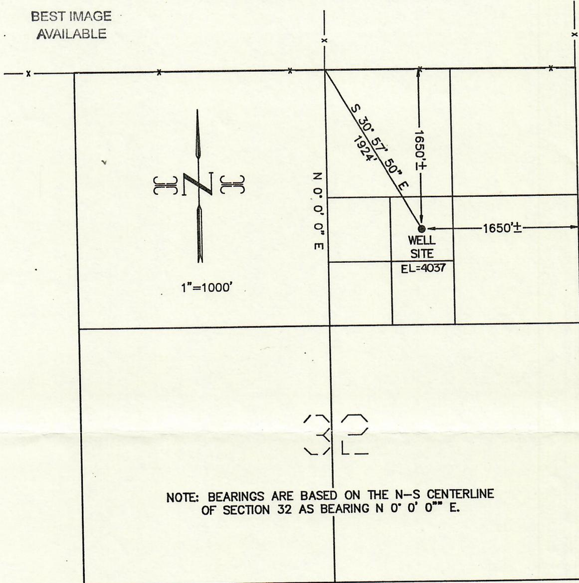
NOTE: BEARINGS ARE BASED ON THE N-S CENTERLINE OF SECTION 32 AS BEARING N 0° 0' 0" E.
