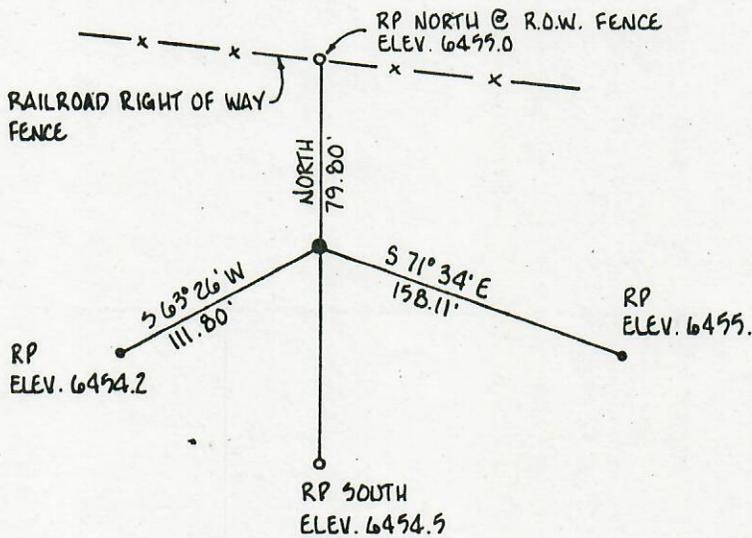
MAP OF WELL SITE TOW CREEK 18-1 LOCATED IN THE NE 1/4 NE 1/4 SECTION 18, T6N R86W OF THE 6TH. P.M. ROUTT COUNTY, COLORADO.
