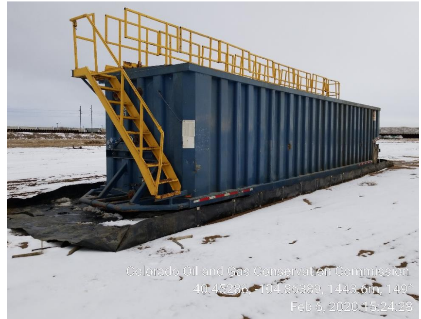
Photo 18: Tank NOT grounded, containment in disrepair
