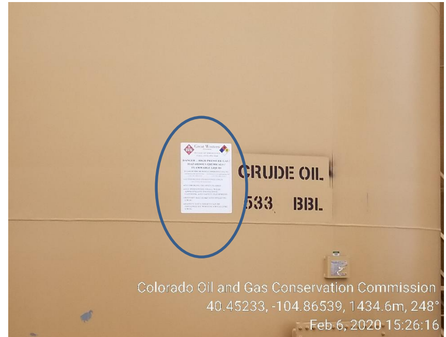
Photo 22: NFPA placard applied to tank
