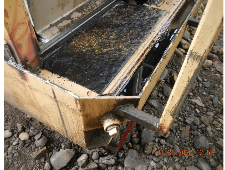
Drip trough along edge of compressor skid is almost full.
